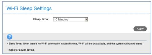
• If there is no Wi-Fi traffic detected then the device will switch off Wi-Fi as determined by the Wi-Fi sleep setting.
