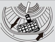
5. Clean the condenser filter after each dry cycle (Fig. 8-14).
