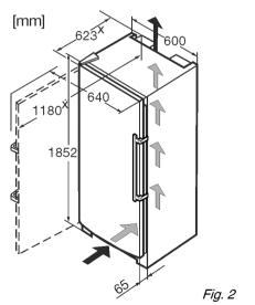
$^{\rm x}$  For appliances supplied with wall spacers, the measurement increases by 35 mm (see 4.2) .
