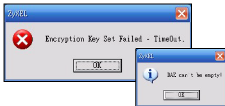
Figure 30 Incorrect DAK or No DAK
