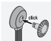
Align the button pin with the strap connector ring and press until it clicks.
