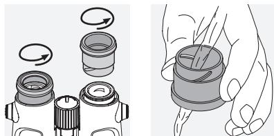
In the event of hard-to-remove dirt (e.g. sand) the eye cups can be unscrewed and cleaned easily.
