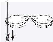
To attach the eyepiece cover, first pull the strap through the loop of the cover.
