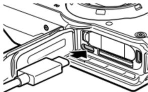
**4** Connect the USB cable to the USB port of the computer.
