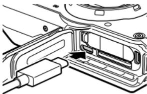
**3** Connect the USB cable to the USB power adapter.
