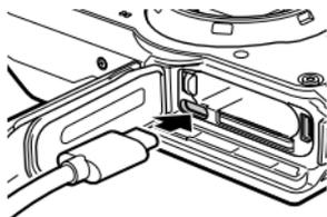
**4** Connect the AC plug cord to the AC adapter, and plug the cord into the power outlet.
