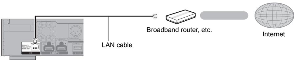
Use category 5e or above straight LAN cables (STP) when connecting to peripheral devices.
