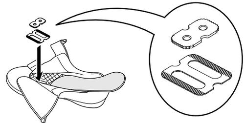
3. From the bottom of the shoe, put a cleat in position over the cleat holes and then a cleat adapter. Be sure the single arrow on the cleat points toward the toe of the shoe. Tighten the cleat mounting bolts (2.5 N·m).
