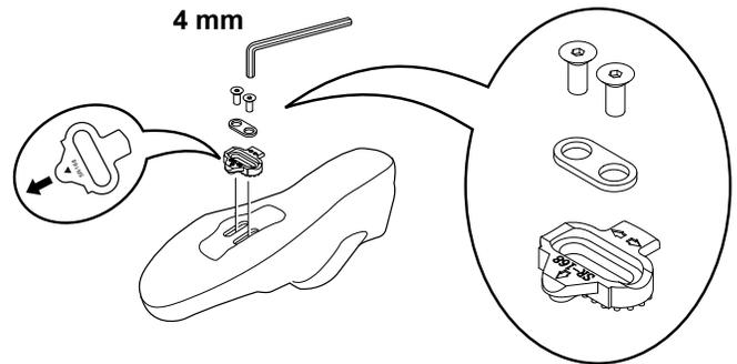
4. The cleat has an adjustment range of 20mm front to back and 5mm left to right. Practice engaging with the Pedal and releasing, one shoe at a time. Readjust to determine the best cleat position.
