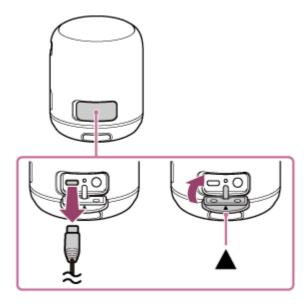
The CHG (charge) indicator lights up in orange while charging. Charging is completed in about 4 hours and 30 minutes\* and the indicator turns off.
