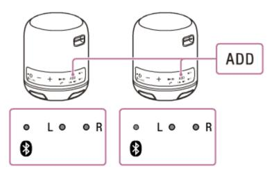
When a connection with the Speaker Add function is established, the L (Left)/R (Right) indicator on both speakers stays lit and the power/ (BLUETOOTH) indicator on either of the speakers turns off.
