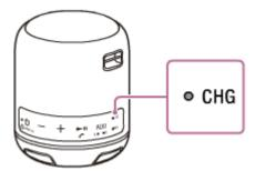
When an abnormality of the built-in battery has been detected, stop charging immediately, wait for a while, and then charge the built-in battery again. If the problem persists, contact your nearest Sony dealer.
