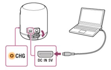
When charging is completed, make sure that the side with the  $\triangle$  mark faces up, and then close the cap securely. The cap plays a very important role in maintenance of the waterproof and dust proof performance.
