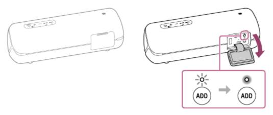
When a connection with the Speaker Add function is established, the ADD (Speaker Add) indicator on both speakers stays lit and the \ (BLUETOOTH) indicator on either of the speakers turns off.
