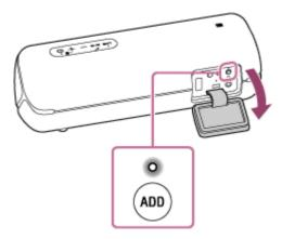
When you press and hold the ADD (Speaker Add) button, the voice guidance outputs from the speaker, then the mode changes.
