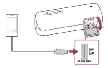
When you connect the speaker to an AC outlet, the connected USB device starts to be charged automatically. If the speaker is being powered by the built-in battery only, proceed to step ②.
