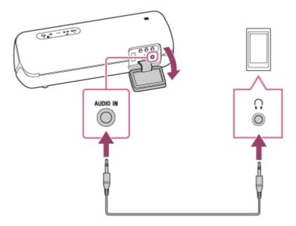
\*1 If you use an audio cable (with stereo mini plugs) with significant resistance, the sound may be lower. Therefore, make sure you use a cable (with stereo mini plugs) without resistance.
