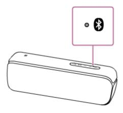
Perform the pairing procedure on the BLUETOOTH device to detect the speaker.
