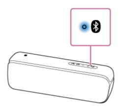
The speaker has been connected to the BLUETOOTH device.
