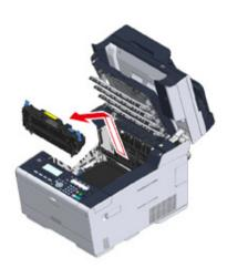
Turn the lock levers (g) on the both sides of the belt unit toward you and remove the belt unit by holding the lock levers.
