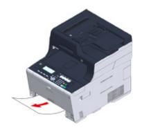
If jammed paper cannot be found, check the positions of the paper guides and paper stopper in the cassette and ensure that paper is correctly loaded.
