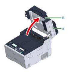
3 Press the button (A) and open the output tray (d) completely.
