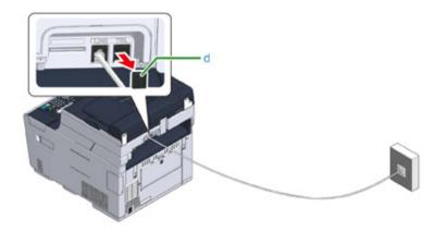
Plug the telephone cable (f) that is connected to the external telephone into the TEL connector (e) of the machine.
