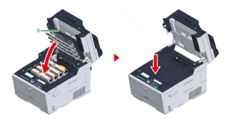
Hold the handle (B) to close the scanner unit (c).
