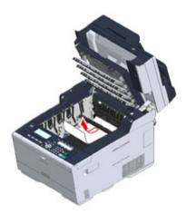
11 Hold the fuser unit handle and place the fuser unit into the machine.
