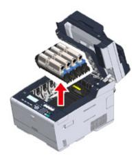
5 Cover the removed image drums with paper so that the image drums are not exposed to light.
