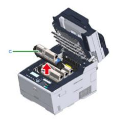
Hold the cartridge, pinch the tip of blue lever (d) of the toner cartridge, and turn it toward you until the tip aligns on the lug of the cartridge.
