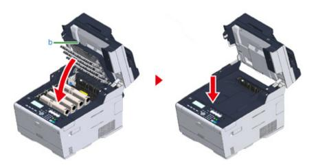
16 Hold the handle (B) to close the scanner unit (a).
