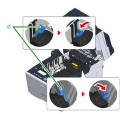
Hold the fuser unit handle and lift the fuser unit out of the machine.
