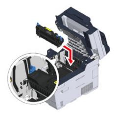
15 Tilt the lock levers (f) on the both sides of the fuser unit.
