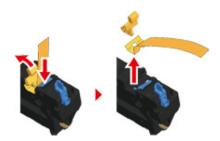
Hold the fuser unit handle and aligning the fuser unit to the grooves behind the toner cartridges, place the fuser unit into the machine.
