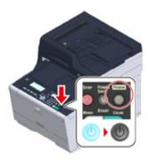
The "System moves to shutdown. Please confirm status when status LED is blinking." message is displayed on the operator panel, and the power switch LED lamp flashes at approximately one-second intervals.
