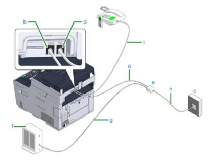
Plug one end of the included telephone cable (a) into the LINE connector (b) of the machine and the other end into a phone line splitter (e).
