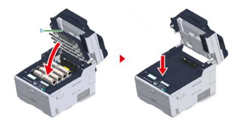
7 Hold the handle (B) and close the scanner unit (a).
