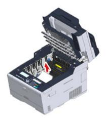
If paper jams in the fuser unit, press the jam release lever (c) on the fuser unit and slowly pull the jammed paper toward you.
