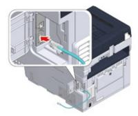
Pass the LAN cable under the tab, and then close the interface cover.
