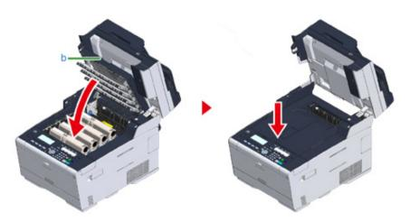
Hold the handle (B) to close the scanner unit (a).
