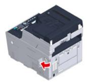
✓ Insert one end of the LAN cable into the network interface connector.
