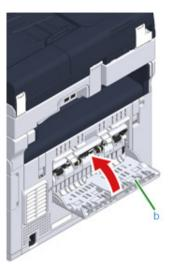
Hold the handle (B) and open the scanner unit (c) completely.
