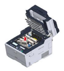
Hold the cartridge, pinch the tip of blue lever (c) of the toner cartridge, and turn forward until the tip aligns on the lug of the cartridge.
