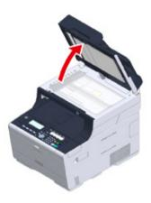
Wipe lightly the document holding pad (a) and document glass (b) with a soft cloth that has been slightly moistened with water and squeezed well.
