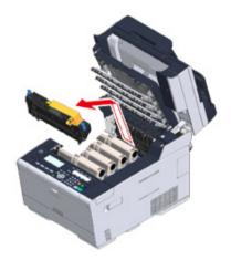
9 Push the blue lever on the fuser unit and remove the orange safety stopper and film.
