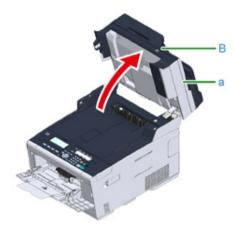
4 Press the button (A) and open the output tray (b) completely.
