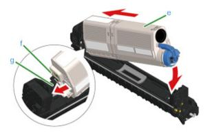
Hold the cartridge, pinch the tip of blue lever (d) of the toner cartridge, and turn forward until the tip aligns on the lug of the cartridge.
