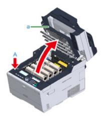
Pinch the tip of blue lever of the toner cartridge and turn forward until the tip aligns on the lug of the cartridge.
