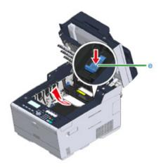
? Tilt the lock levers (f) on the both sides of the fuser unit toward you.
