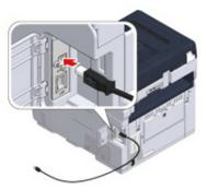
Pass the USB cable under the tab, and then close the interface cover.
