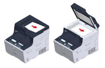
If paper is loaded on the MP tray, remove the paper.
