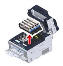
6 Cover the removed image drums with paper so that the image drums are not exposed to light.
