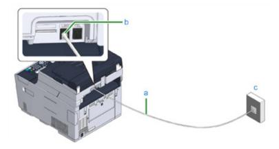
Plug one end of the included telephone cable (a) into the LINE connector (b) of the machine and the other end into a public line (analog) (c).
