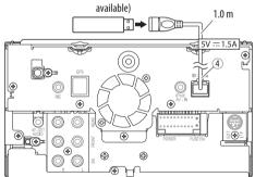
iPod/iPhone (Lightning • Connect the USB extension cable (④) beforehand. connector models) (See the left column.) (commercially available) iPod/iPhone (30-pin connector models) (commercially available) KCA-iP103 (optional accessory) (0.8 m KCA-iP102 (optional accessory) (0.8 m) ٠ 1.0 m \_\_\_\_\_ 5V --- 1.5A ۲ ٠  $\bigcirc$ ۲
