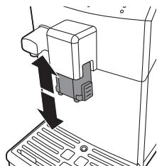
The machine can be used to dispense different coffee types in cups or glasses of different sizes. To adjust the height of the coffee dispensing spout to the size of the cup or glass, slide the spout up or down.
