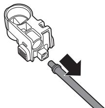
**5** Remove the tube with the fitting.
