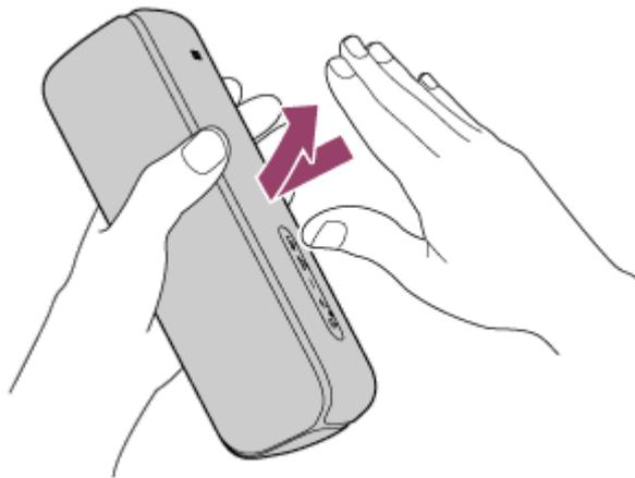
The surface where sound effects are output when you tap are the top, front, both sides, and bottom of the speaker.
