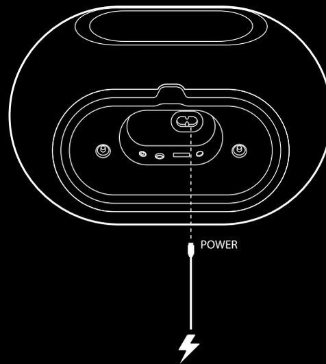
Connect the supplied AC power cable to this input.
