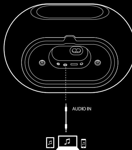
You can connect an analog audio device to the speaker via a 3.5 mm Aux cable.
