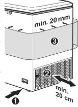
Standard EN 378 specifies that the room in which you install your appliance must have a volume of 1 m<sup>3</sup> per 8 g of R 600a / R 290 refrigerant used in the appliance, so as to avoid the formation of inflammable gas/air mixtures in the room where the appliance is located in the event of a leak in the refrigerant circuit. The quantity of refrigerant used in your appliance is indicated on the type plate.
