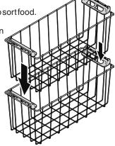
Press the handle downwards, lift and tilt inwards.
