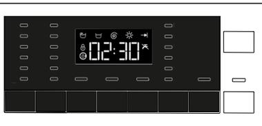
If the water level in the machine is suitable when you press **Start / Pause** button, "Loading door locked" light on the panel is turned off. If the water level in the machine is not suitable when you press **Start / Pause** button, the panel will indicate that the loading door is locked.
