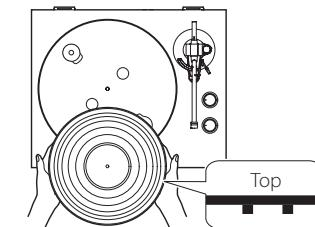
● The rubber mat has a top and a bottom. As shown in the illustration, the side with the ridged concentric circles should be placed down.
