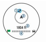
The destination indicator ① shows the direction of your destination relative to the direction you are moving ②. When the destination indicator appears at the top of the circle, you are heading towards your destination. The remaining distance to your destination ③ appears below the circle. The progress bar ④ shows your progress towards your destination.
