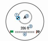
The destination indicator ① shows the direction of your destination relative to the direction you are moving ②. When the destination indicator appears at the top of the circle, you are heading towards your destination. The remaining distance to your destination ③ appears below the circle. The progress bar ④ shows your progress towards your destination.
