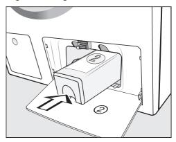
■ Push the **UltraPhase 2** detergent cartridge into **compartment** ② until it locks into position.
