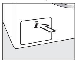
■ Press the drain pump access panel.
