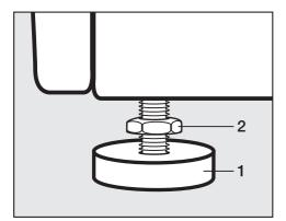
■ Using the spanner supplied turn counter nut 2 in a clockwise direction. Then turn counter nut 2 together with foot 1 to unscrew.
