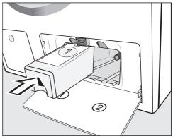
■ Push the **UltraPhase 1** detergent cartridge into **compartment** ① until it locks into position.
