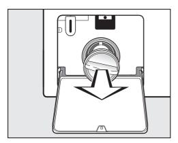
Remove the drain filter completely.
