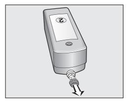
Remove the stopper from the detergent cartridge.
