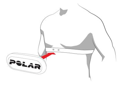
① Detach the connector from the strap and rinse the strap under running water after every use. Sweat and moisture may keep the electrodes wet and the heart rate sensor activated. This will reduce the transmitter battery life.
