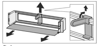
Fig. 6The door racks can be dismantled for cleaning.
