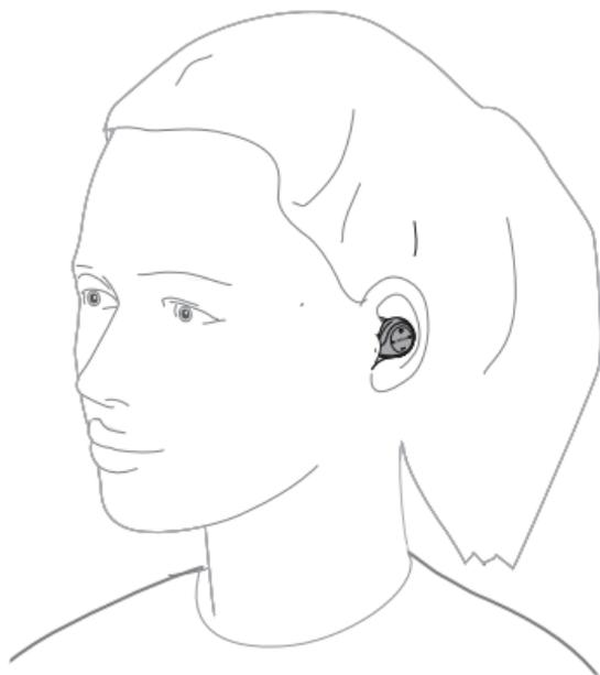
The top of the EarWing should fit tight into the ridge of the ear.
