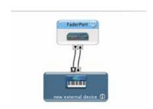
3. Drag the in / out virtual patch cords to hook FaderPort up to the new external device just added. Close the Audio MIDI Setup window.
