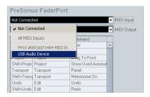
3. In the FaderPort Configuration menu to the right, set both the MIDI Input and the MIDI Output to "USB Audio Device" (PC) or "PreSonus FaderPort (Mac)
