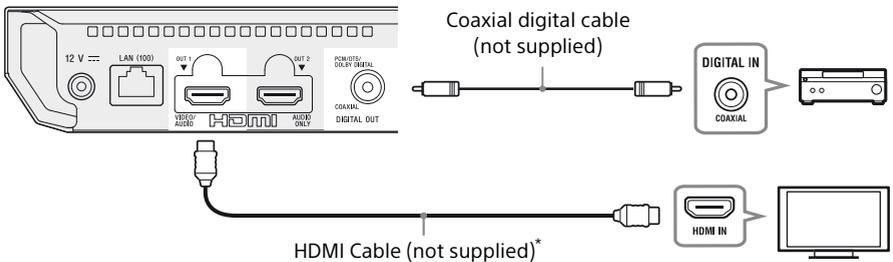
\* Premium High Speed HDMI Cable or High Speed HDMI Cable that supports 18 Gbps bandwidth.
