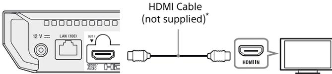
\* Premium High Speed HDMI Cable or High Speed HDMI Cable that supports 18 Gbps bandwidth.
