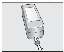
■ Remove the cap from the cartridge.
