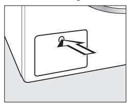
■ Press the drain pump access panel.
