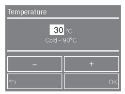
The numerical value is highlighted in white. Touching the – sensor decreases the value and touching the + sensor increases it. The OK is used to adopt the selected value.
