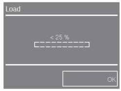
The display shows the amount of laundry loaded in the drum as a % (in 25% steps) of the maximum load permissible for the programme selected.
