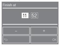
■ Use the + and - sensors to set the hour and confirm with the OK sensor.
