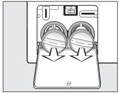
■ Remove the drain filters completely.
