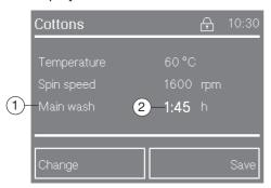
The washing machine lets you know which section of the programme has been reached ① and the programme duration remaining ②. If a delay start time has been selected, then this will appear in the display.
