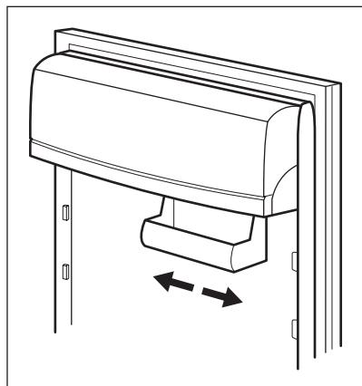
The model is equipped with a variable storage box which is fitted under a door shelf compartment and can be slide sideways.
