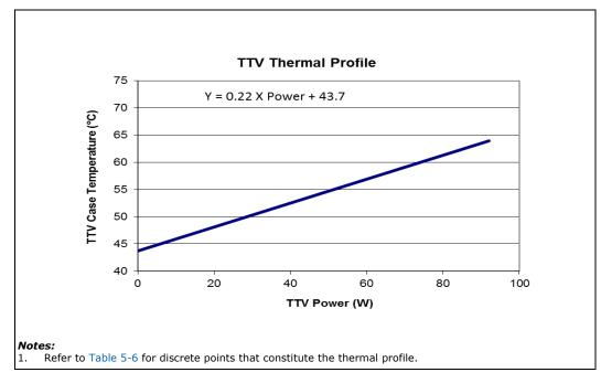
Table 5-6. Thermal Test Vehicle Thermal Profile for PCG 2015D Processor (Sheet 1 of 2)
