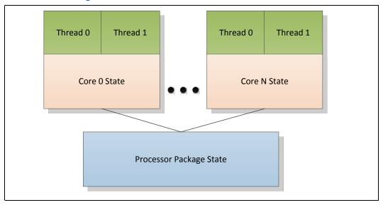
While individual threads can request low-power C-states, power saving actions only take place once the processor IA core C-state is resolved. processor IA core C-states are automatically resolved by the processor. For thread and processor IA core C-states, a transition to and from C0 state is required before entering any other C-state.
