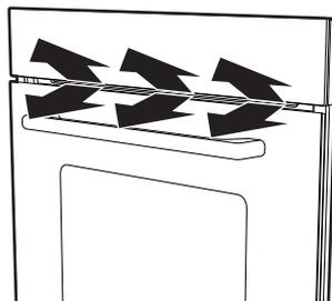
The fan cools the oven and comes into operation during cooking.
