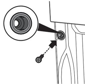
Cover the bushings with the covers removed previously.
