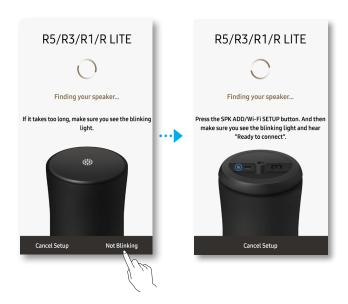
WAM5500/WAM3500/WAM3501/WAM1500/WAM1501/ WAM1400: On the lower part of the speaker, briefly press SPK ADD/Wi-Fi SETUP and start Wi-Fi Setup.
