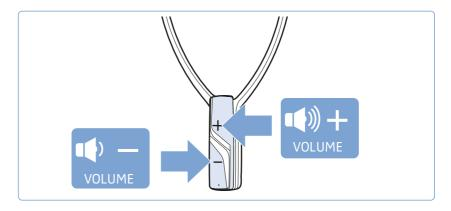
If you have set a very high volume level and switch the stethoset receiver off and on again, the volume is reset to a moderate level to protect your hearing.
