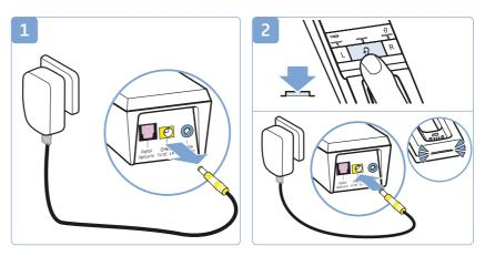
The protected settings mode is activated. The *Transmitter status* LED flashes blue. The LED segments indicate the current settings as specified in the following chapters:
