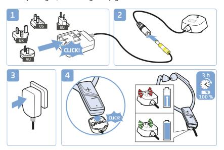
You can also use the stethoset receiver during charging. Please note, however, that the receiver can get slightly warm during charging. The charge status of the rechargeable battery is displayed on the transmitter (see page 16).
