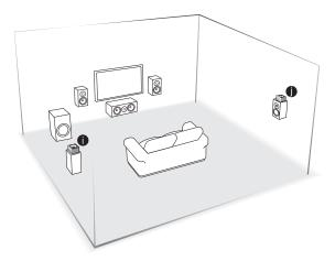
Change the setting: Press RCV and then HOME on the remote controller, select "Setup" - "2. Speaker Setup" - "Speaker Settings" and set "Height Speakers Type" to "Dolby Enabled Speaker (Surround)" as shown in the figure.
