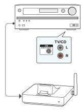
Connect an Onkyo component with RI jack to this unit using an RI cable and an analog audio cable. For details, refer to the instruction manual of the component with RI jack. The RI cable can be connected in any order. When there are two RI jacks, both jacks work in the same way and are interchangeable.
