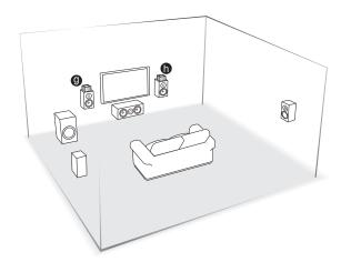
Change the setting: Press RCV and then HOME on the remote controller, select "Setup" - "2. Speaker Setup" - "Speaker Settings" and set "Height Speakers Type" to "Dolby Enabled Speaker (Front)" as shown in the figure.
