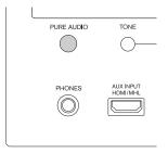
Selecting Pure Audio for listening mode turns off the power to the display and analog video circuitry, but the video signals input through HDMI input are output from HDMI output.
