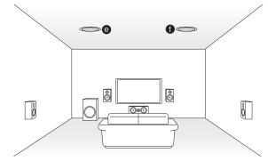
Change the setting: Press RCV and then HOME on the remote controller, select "Setup" - "2. Speaker Setup" - "Speaker Settings" and set "Height Speakers Type" to "Top Middle".
