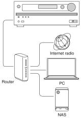
To stream a music file, you need a NAS device with DLNA server functions or a PC where a player (e.g., Windows Media® Player 11 or12) with DLNA server functions is installed. To enable streaming with Windows Media® Player 11 or 12, you must first configure the settings.
