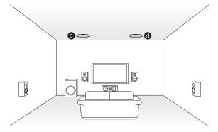
Change the setting: Press RCV and then HOME on the remote controller, select "Setup" - "2. Speaker Setup" - "Speaker Settings" and set "Height Speakers Type" to "Top Front" as shown in the figure.
