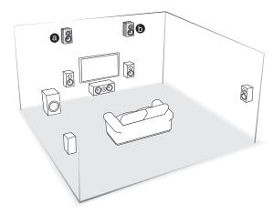
Change the setting: Press RCV and then HOME on the remote controller, select "Setup" - "2. Speaker Setup" - "Speaker Settings" and set "Height Speakers Type" to "Front High".
