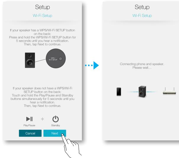
**4** Once an available device is found, the product tries to connect to the newly found smart device first, then it attempts to connect to the wireless network. In case of secure network, the password prompt appears on the smart device screen. Use the onscreen keyboard to enter the password.
