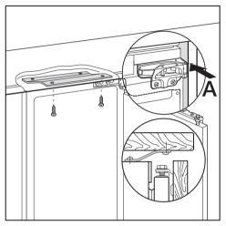
■ Use chipboard screws (4 x 19 mm) to secure the appliance to the worktop through the mounting plate, as shown.
