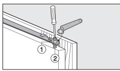
Whilst counterholding adjusting bolts
