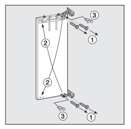
■ Remove screws ①, and use stoppers supplied ③ to plug the empty holes.
