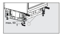
Adjust both rear feet using appropriate screws ① at the front right and left in the appliance plinth. Use a 7 mm flat-bladed screwdriver to do so.
