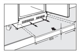
If there is a continuous plinth in the kitchen, a ventilation gap will need to be made in the plinth for the appliance:
