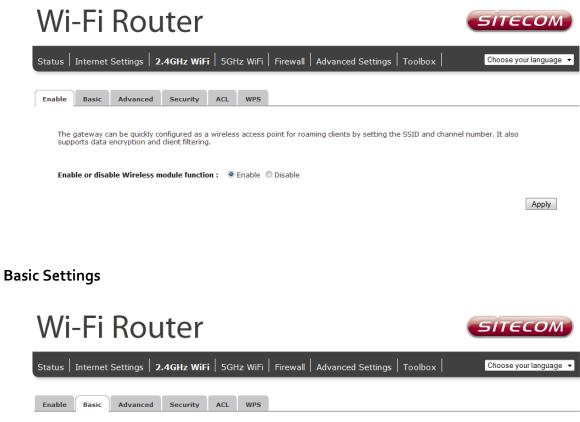
This page allows you to define ESSID, and Channel for the wireless connection. These parameters are used for the wireless stations to connect to the Access Point .
