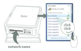
• Fill in the password for the wireless network. The correct password can be found on the sticker on the bottom of the router, or in the Network Details Folder.
