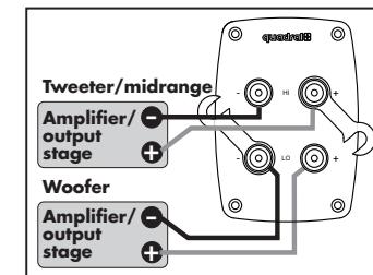
In the biwiring/biamping mode, the bass frequencies are controlled via the two lower terminals – and the midrange/treble frequencies via the two upper terminals. Make sure you use the correct polarities in these modes and that you remove the jumpers on the speaker terminal to avoid damaging your amplifier.
