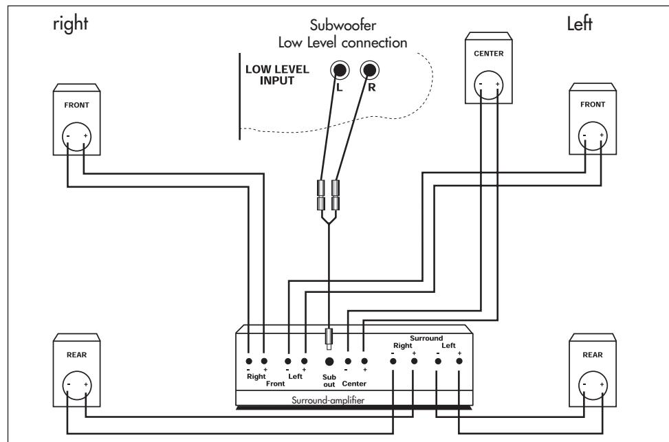
Once you have positioned and connected your speakers as shown in the illustration, you should perform the necessary settings in the bass management system of your surround amplifier. Make sure you read the user manual supplied by your amplifier's manufacturer before doing this.
