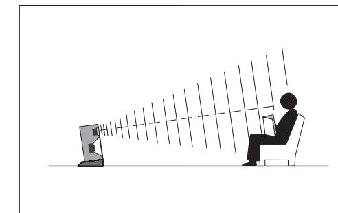
loud wall reflections, the distance from the side walls of the room can even be 50 cm or more. Bookshelf speaker units sound best on a speaker stand or shelf, with the tweeters arranged at ear height. The cases should be angled and slightly tilted to achieve this. So far as possible, the speakers should be equidistant from the listening position, while the distance of the speakers from each other can be rather less than the distance from the listener.
