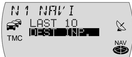
Press the **NAV** button (1) once to switch from the radio or CD-changer (optional) audio source to the main navigation menu.
