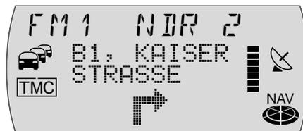
**Note: You now have the option of storing the destination using buttons 1 - 6 (14). To store it, press and hold down the relevant button for longer than two seconds.**
