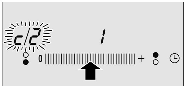
5. Press and hold the  $\Theta$  symbol for more than 4 seconds until a beep sounds to confirm this. The settings have been correctly stored
