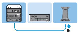
Connect an additional identical audio cable to the output ("OUT") on the transmitter and to the input ("IN") on the amplifier.
