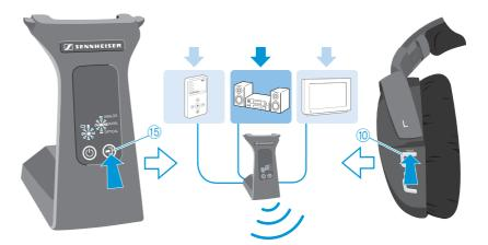
Touch the touch key for selecting the audio source (5) on the transmitter or press the Input button (0) on the headphones.
