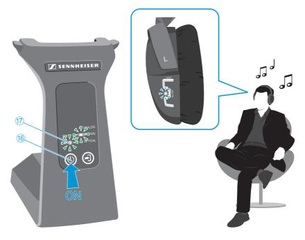
If the transmitter doesn't receive an audio signal for more than 3 minutes, it switches, depending on the setting, to either standby mode or loop through mode. If the transmitter receivers an audio signal within the next 10 minutes, it automatically switches on again.
