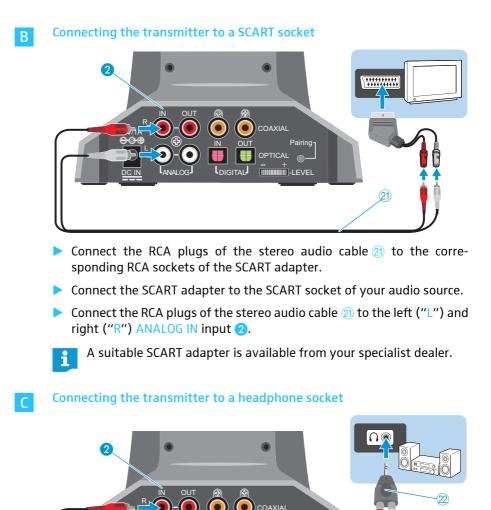
Connect the RCA plugs of the stereo audio cable 21 to the corresponding RCA sockets of the audio adapter 22.
