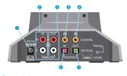
1 DC IN socket for power supply unit
