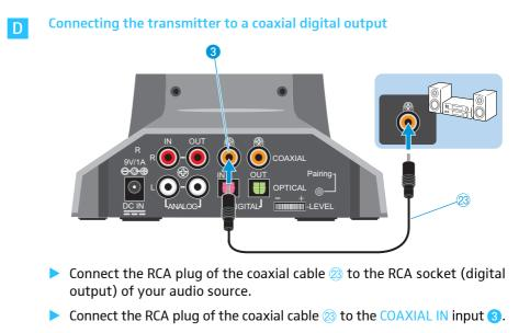
Connecting the transmitter to a coaxial digital output
