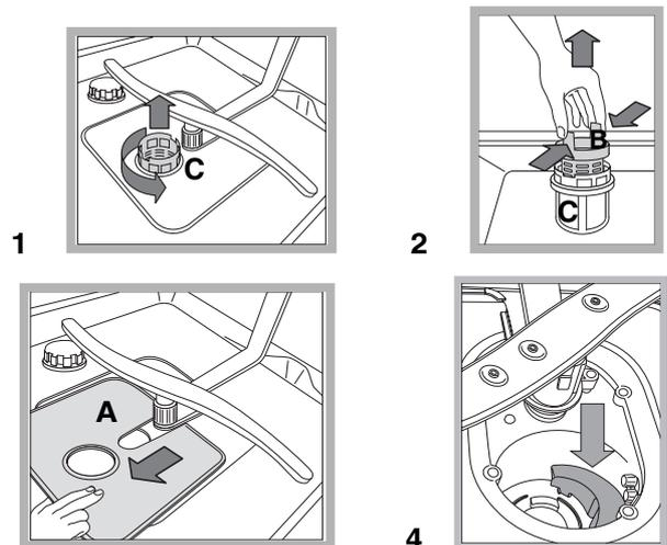
After cleaning the filters, replace the filter assembly and fix it in position correctly; this is essential for maintaining the efficient operation of the dishwasher.
