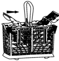
Movement required to extract the inserts
