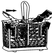
Movement required to extract the inserts
