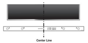
2. Align the Wall Mount Guide's Center Line with the center of your TV (if you are mounting the Soundbar below your TV), and then fix the Wall Mount Guide to the wall using tape.
