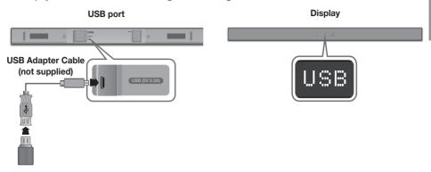
1. Connect a USB adapter cable with a male USB 2.0 Micro USB plug (Type B) on one end and a standard female 2.0 USB jack (Type A) on the other end to the micro USB jack on your Soundbar.
