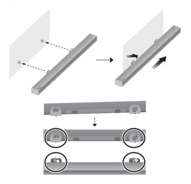
Install the Soundbar with the attached Bracket-Wall Mounts by hanging the Bracket-Wall Mounts on the Holder-Screws on the wall.
