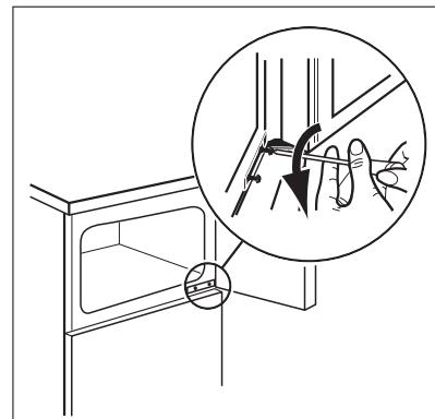
3. Remove the doors by pulling them slightly and remove the hinge.
