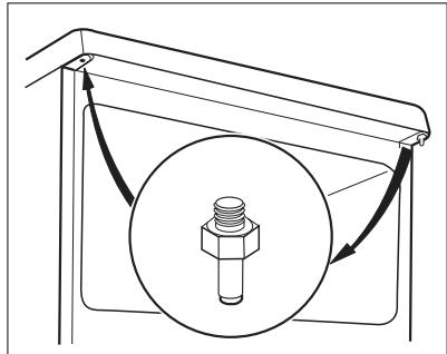
9. Fit the doors into the pins and install the doors. Install the hinge.
