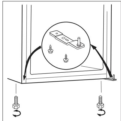
6. Unscrew the bottom far side screw and install on the opposite side.
