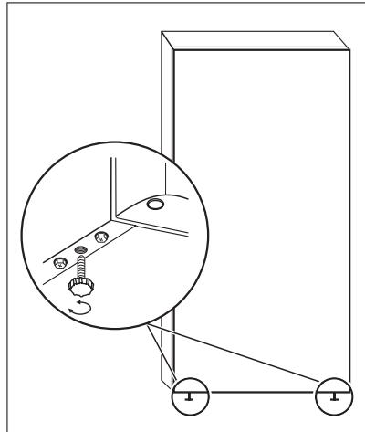
When placing the appliance ensure that it stands level. This can be achieved by two adjustable feet at the bottom in front.
