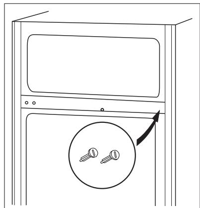
5. Unscrew both adjustable feet and the screws of the bottom door hinge. Remove the bottom door hinge and install it on the opposite side.
