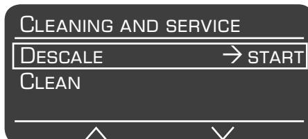
The **start** button 8 flashes while the different descaling processes are running. The figures on the top right indicate the progress of the program.
