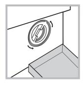
Position a container collecting the drained water (approximately 1.5 l) correctly (see figure);
