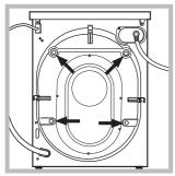
2. Remove the 4 transit bolts used during transportation and the corresponding spacers on the back of the machine (see figure).
