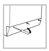
1. Remove the kick strip on the front of the machine using a screwdriver (see figure);
