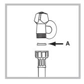
2. Place the seal A (provided in the bag) on the end of the inlet hose and screw it to a cold water tap with a 3/4 BSP threaded connection (see figure).
