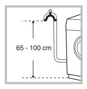
Connect the outlet hose to a draining duct or a stand pipe at a height between 65 and 100 cm from the floor. Do not bend it under any circumstances.
