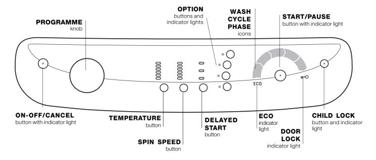
**ON-OFF/CANCEL** button with indicator light  $\circlearrowleft$ : press the button briefly to switch the machine on or off. The green indicator light shows that the machine is switched on. To switch the washing machine off during a wash cycle, press and hold the button for approximately 2 seconds; pressing the button quickly or accidentally will not switch the machine off. If the machine is switched off during a wash cycle, the programme will be cancelled.
