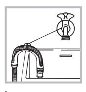
Alternatively, place the end of the hose over the edge of a washbasin or tub, fastening the hose supplied to the tap (see figure).
