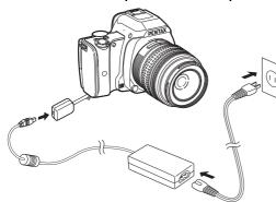
Connect the AC adapter to the AC plug cord, and plug the cord into the power outlet.
