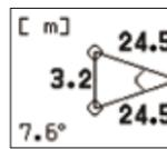
When the measurement is successful, you see the height from the base to the top displayed on the internal LCD with Hgt + Hgt2 (solid). For more information, refer to the external LCD. "Base" and "Top" can be switched.
