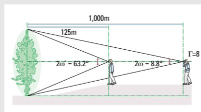
Referring to the ISO 14132-2:2002 standard that was established at the same time as the abovementioned ISO 14132-1:2002, binoculars that provide an apparent field of view over 60° are considered wide-viewfield binoculars.
