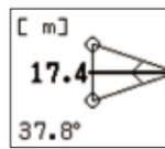
When three-point measurement is achieved, the height between points 2 and 3 is displayed on the internal LCD with Hor Hgt+Hgt2 (solid), and Hgt(2) and Ang(2) are shown on the external LCD. Points 2 and 3 can be reversed.
