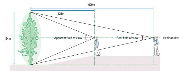
\* Apparent field of view is calculated based on the ISO 14132-1:2002 standard. For details, see p 54.
