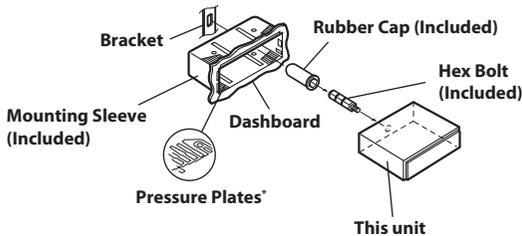
\* If the installed mounting sleeve is loose in the dashboard, the pressure plates may be bent slightly to remedy the problem.
