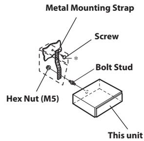
\* For the screw\*, provide a proper screw to the chassis installing location.
