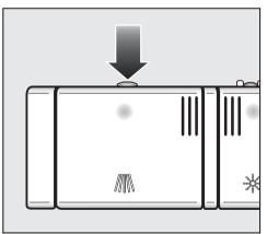
Press the opening catch on the detergent dispenser. The flap will spring open. The flap is always open at the end of a programme.
